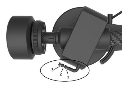
Hang the loop of the thread of the anti-skating weight in the groove of the anti-skating stub (9) corresponding to the downforce applied to your cartridge and hang the thread in the groove of the wire support (8).
