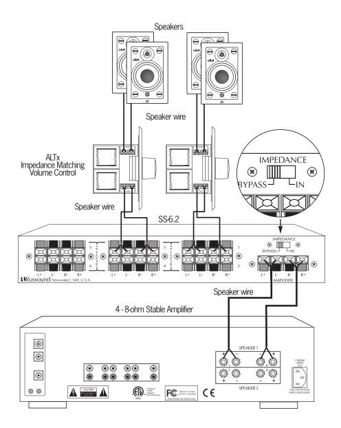
Typical connections with external impedance matching (Impedance switch set to BYPASS)
