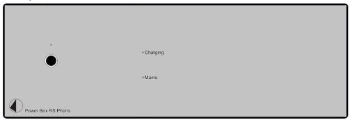
**Toggle switch** on the left side will enable or disable output socket with 2x18V. The blue LED above the switch shows that the socket is active.
