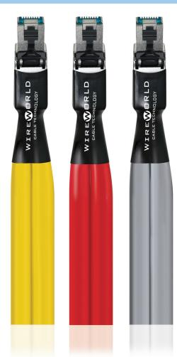
Fireworld Ethernet cables use an innovative flat design to support next generation Category 8 transmission speeds while providing greater flexibility and ease of use than conventional round Ethernet cables. Even though they have full sized 23 gauge conductors and triple-shields on each conductor pair, this patent pending Tite-Shield design is just a tenth of an inch thick. This elegant cable structure also simplifies assembly with Wireworld shielded RJ-45 plugs.
